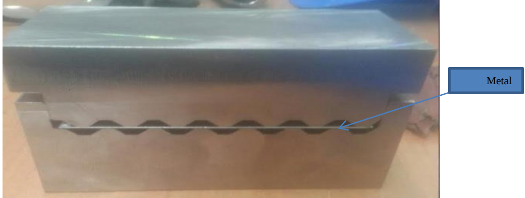
Fig. 2. The mold used in experimental studies and the appearance of the sheet plate placed in the mold
